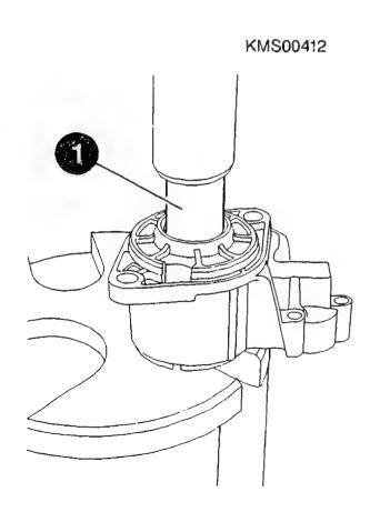
COMPONENT CHECKING AND REPAIR Checking drive-end shield (version with bushing) After removing radial lip-type oil seal and bushing, use three-square scraper to carefully remove projecting
